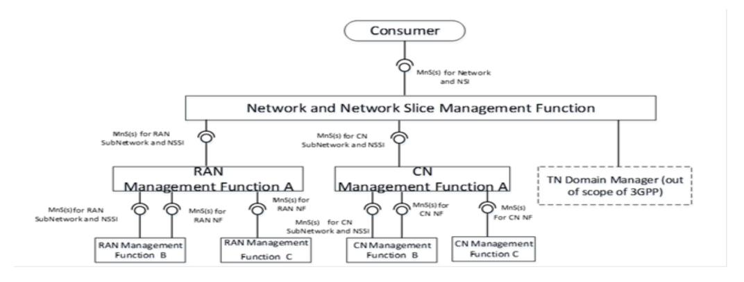
An example of deployment scenario for management of a mobile network including network slicing
