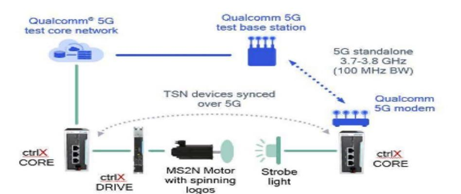
Qualcomm 5G test network and 5G industrial test device with 5G modem
