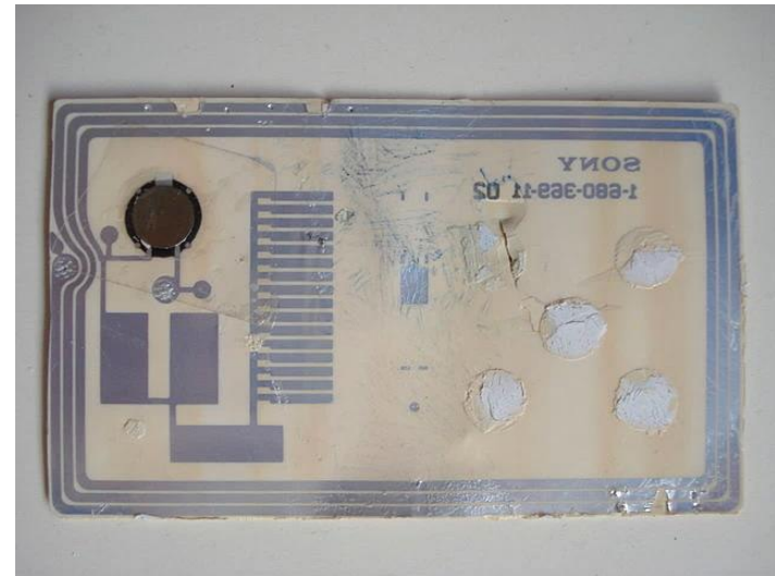
A defaced FeliCa (EZ-Link) card, revealing its internal circuitry.
