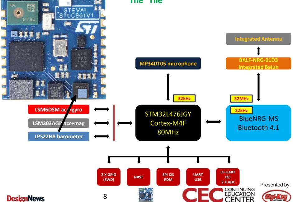
The "Tile" STLCSOLVI **Integrated Antenna BALF-NRG-01D3 MP34DT05** microphone **Integrated Balun** 32kHz 32MHz LSM6DSM acc+gyro 32kHz STM32L476JGY BlueNRG-MS LSM303AGR acc+mag Cortex-M4F Bluetooth 4.1 80MHz **LPS22HB** barometer **LP-UART** 2 X GPIO SPI 12S **UART NRST** I2C (SWD) PDM **USB** 2 X ADC Presented by: CONTINUING EDUCATION 9 **DesignNews**
