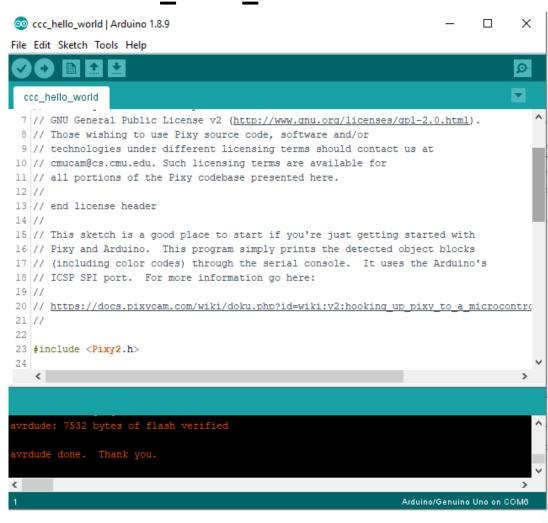
This sketch is a good place to start if you're just getting started with Pixy and Arduino.This program simply prints the detected object blocks (including color codes) through the serial console It uses the Arduino's ICSP SPI port.
