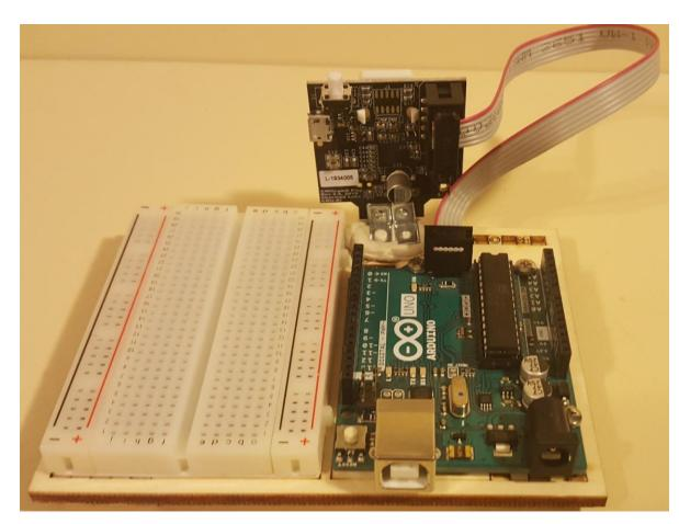
Attaching ribbon cable to the Pix2y camera and the Arduino
