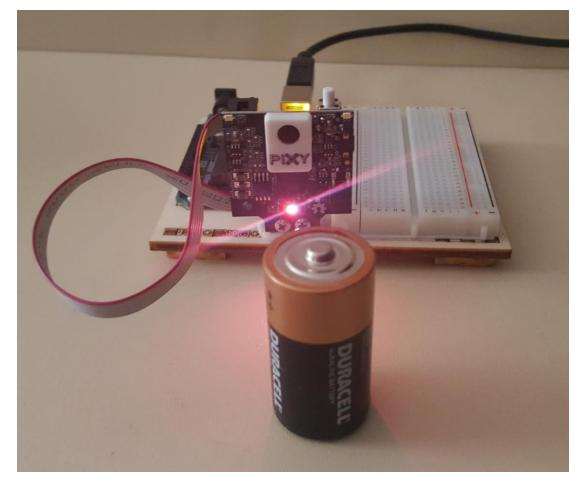
RGB turns on when object is detected by the Pixy2 camera smart sensor
