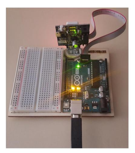
USB powering of the Pix2y camera through an Arduino
