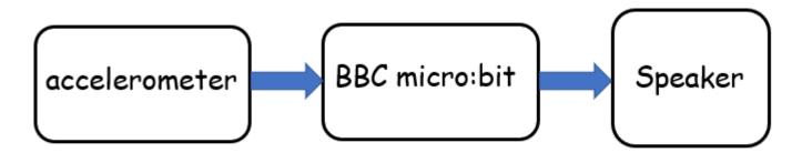
Talking Accelerometer Gesture Device Block Diagram
