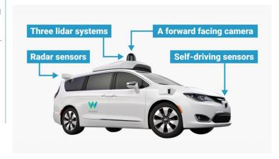
**LIDAR:** Laser Imaging Detecting And Ranging
