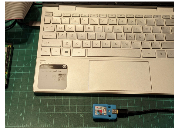
UNITV Camera Attached to COM Port
