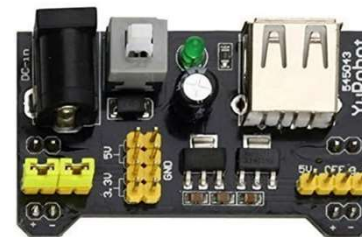
Solderless Breadboard Power Supply Module with 9V Battery Clip Power Cable
