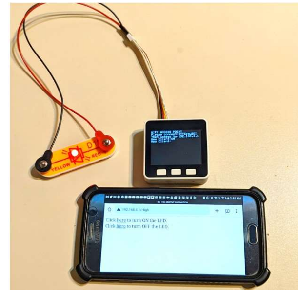
Web Server-Controller in operation
