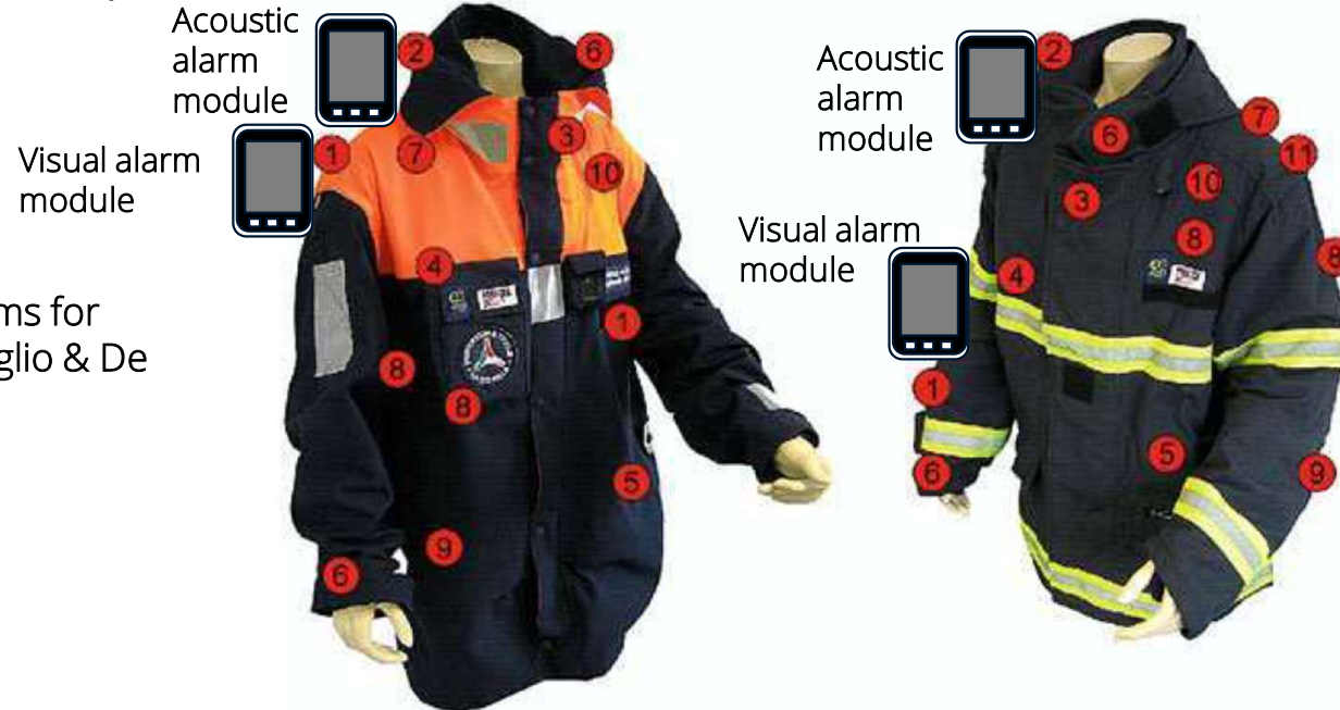
1-Visual alarm module (1x in the FF OG, 2x in the CP OG); 2-acoustic alarm module; 3-external temperature sensor; 4-Wi-Fi communication module; 5-Professional Electronic Box (PEB); 6-triaxial accelerometers (2x); 7-GPS module; 8-Flexible antenna (2x); 9-Flexible battery; 10-CO sensor; 11-Heat flux sensor (only FF OG)
