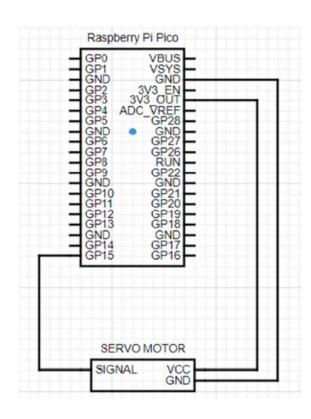
Servo Motor Controller Circuit Schematic Diagram
